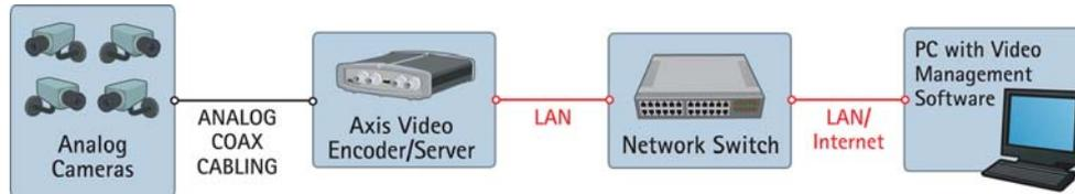
*The video encoder/server migrates the analog cameras into an IP-based video solution*
