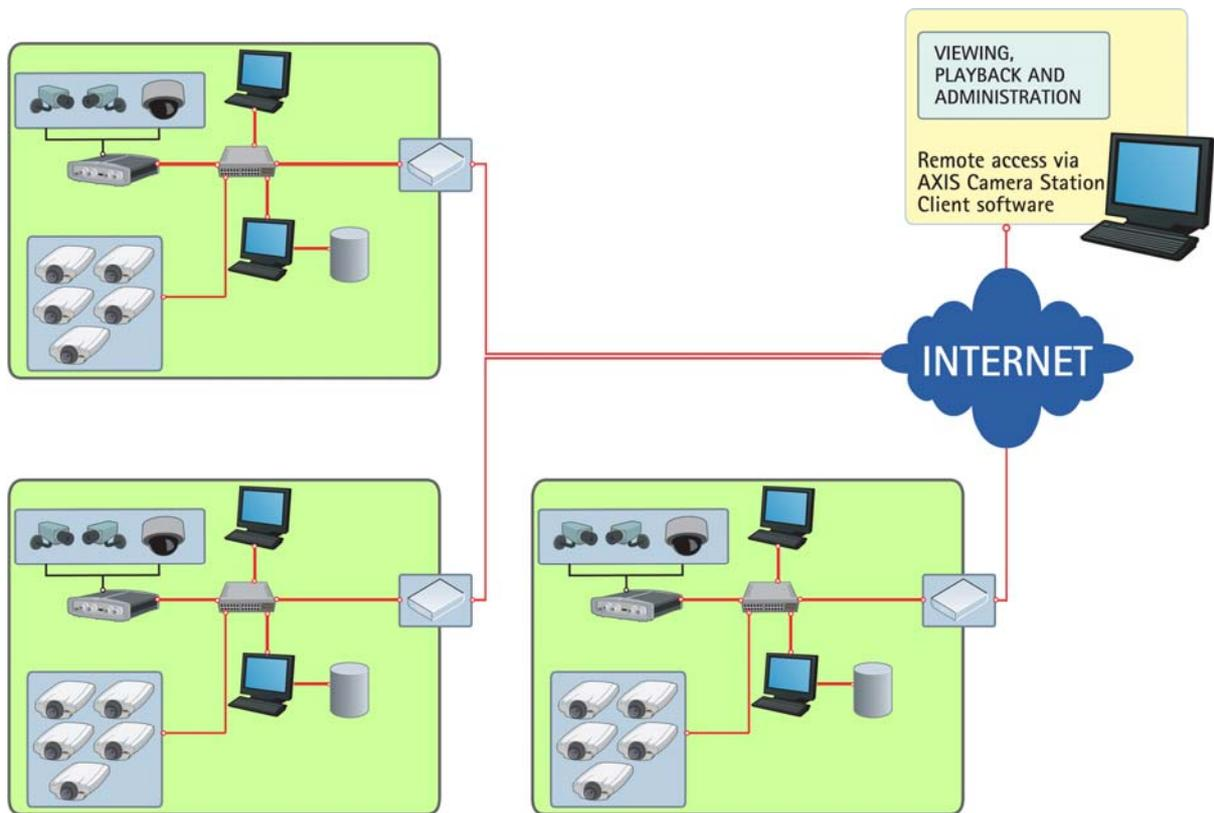
*You can also switch between different AXIS Camera Station servers using the client software*
