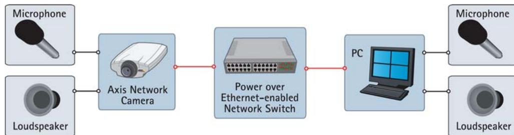
Audio modes may be simplex (audio is sent either by the operator or the camera) or duplex (audio is sent to and from the operator simultaneously). Audio can be compressed and integrated into the video stream, and sent over a network for monitoring and/or recording. There are many audio compression formats. The higher the compression level, the more latency is introduced. If synchronized audio and video is a priority, the preferred compression standard is MPEG.
