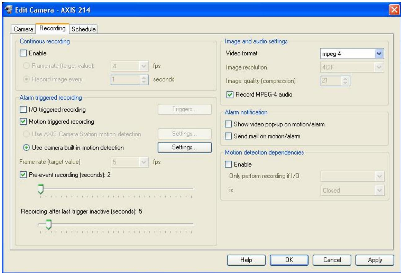
In continuous recording, you can set how many frames per second and how often (i.e. every few seconds between images) the camera should send images to the software for recording. Continuous recording uses more disk space than an alarm-triggered recording.
