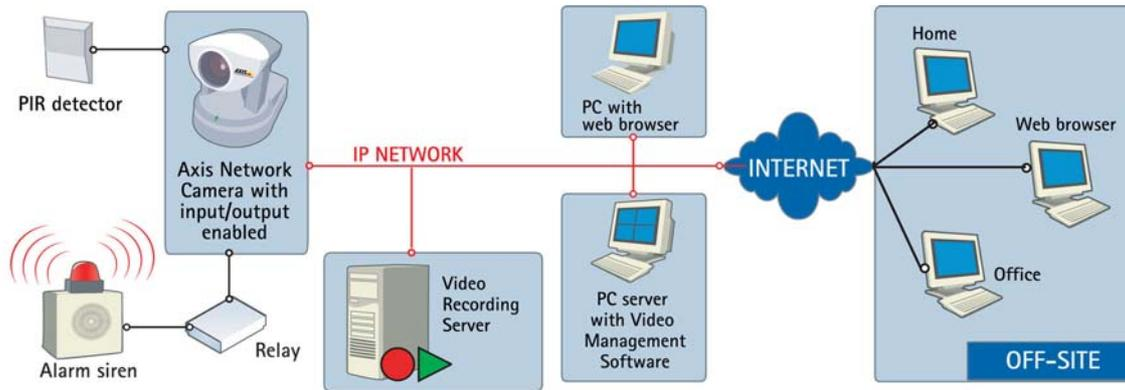
*An IP-Surveillance or network video system with alarm integration*
