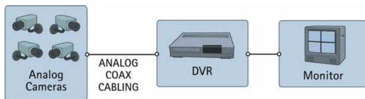
*An analog video system that incorporates a DVR (digital video recorder)*
