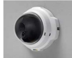
Pan/tilt/zoom (PTZ): The camera's view can be remotely controlled, either manually or automatically, for panning from side to side, tilting up and down, and zooming in and out of an area or object. There are now mechanical as well as non-mechanical pan/tilt/zoom cameras:
