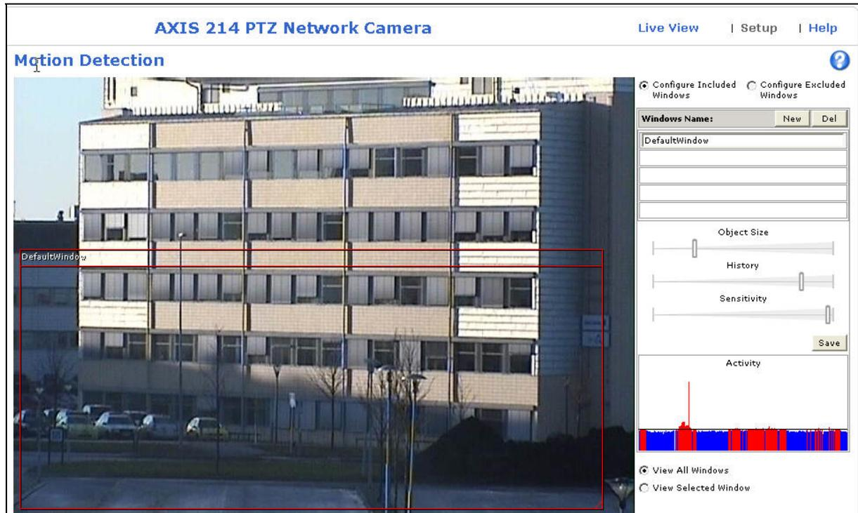
When configuring for video motion detection, you can adjust the size of the window where you want motion to be detected and drag the window to the desired position. You can then adjust sliders for the object size (how large should the object be in order for the trigger to activate), history (how far back in time should the reference point for motion detection be), and sensitivity (how big should a change in the pixels be in order to trigger an alarm).
