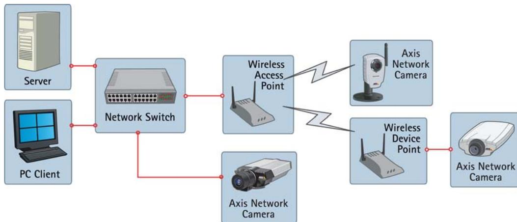
*Network including both wired and wireless connections*
