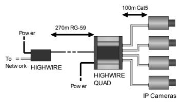
In the example above, the HIGHWIRE QUAD provides all four cameras with both a POE power supply and Fast Ethernet connection, and converts the data into a digital signal that can be carried by the existing coaxial video cable.
