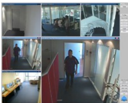
Monitor application. In this example, a 3×3 view with a hot spot is used in the Monitor 's camera layout.
