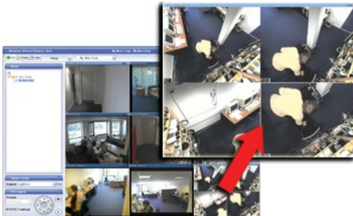
Two by Two: Live tab displaying four different viewpoints from a single IPIX camera; in this example, the IPIX camera's four viewpoints are enlarged for clarity.
