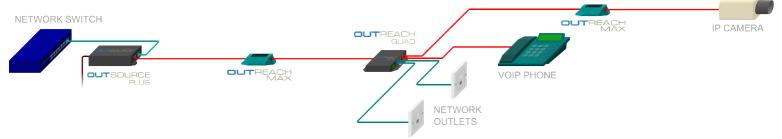
In this example an OUTREACH MAX is used to forward enhanced PoE Plus power to an OUTREACH QUAD PoE-forwarding switch, located up to 200 metres from the network switch and OUTSOURCE PLUS injector.
