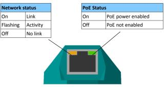
Note that the LEDs on OUTREACH MAX will not light until the PoE source and powered device are *both* connected
